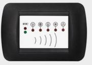
It provides access to the room in different mode for guests, managers, staff and maintenance operators. It is provided with illuminated insertion slot for chip cards with ISO 7816 format and 2 leds for card validity. It is also provided with 5 light signals to display: "guest in room", "do not disturb", "room to clean", "mini-bar to check", "help call/flood".
