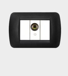
It detects the presence of guests or staff in the room and activates relevant services. Light for easier insertion of jack. It is housed in 1-module box. It is connected to the control unit UGC with 6-wire cable terminated with RJ12 PLUG.
