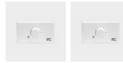
RVI volume controls series is made up of a control circuit with 11 positions switch (10 + off) and a transformer, in order to be used in 70-100V systems. It can be used to set the volume of one or more constant voltage speakers. Available in 3 versions: 30W, 60W or 100W. Thanks to the on board relay (enabled through a 24Vcc control), the volume control can be bypassed and forcibly brought to the maximum volume in case of priority announcements. Set for box 503 mounting.
