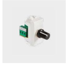
It is necessary when you want to control the volume in a single zone/room, separated from the others. Provided with triple screw terminal, it inserts between signal distribution line and the speakers of a given zone. It is also provided with a switch which opens when the volume control is rotated until zero. The switch, with separated terminals, can be used to stop the power to the amplified speakers when the volume is zero. It occupies 1 unit in civil series.
