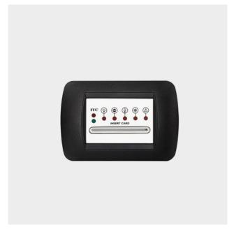
It provides access to the room in different mode for guests, managers, staff and maintenance operators. It is provided with illuminated insertion slot for chip cards with ISO 7816 format and 2 leds for card validity. It is also provided with 5 light signals to display: "guest in room", "do not disturb", "room to clean", "mini-bar to check", "help call/flood".
