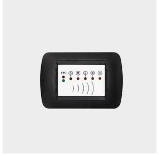
It provides access to the room by proximity cards ISO 7816 format in different mode for guests, managers, staff, maintenance operators, etc. Max. reading distance 5 cm. It is provided with 2 leds for card validity and 5 light signals to display: "guest in room", "do not disturb", "room to clean", "mini-bar to check", "help call/flood alarm".
