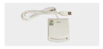
Chip card reader/writer in desktop version, complete with connection cable to PC via USB port. Dimensions: 72x28x84 mm. Weight 0.1 kg.
