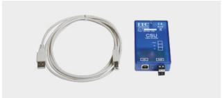
It converts the signal from USB to RS485 half duplex standard. 220Vac, 5VA power supply. 2-ways extractable terminal for bus connection RS485. 3 signal led lights: red – power supply; blue – TX; green – RX. USB connecting cable included (male connector Type B – Type A). Dimensions: 105x25x57. Weight: 0.5 kg.
